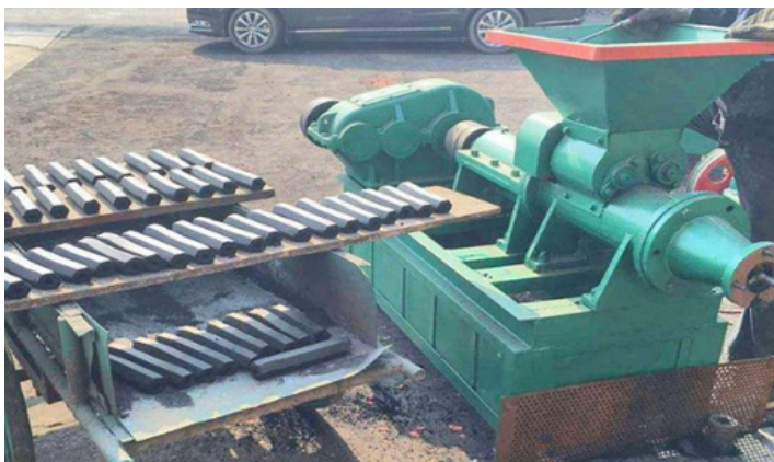
Figure 2.4: Screw Extrusion briquetting machine (making cylindrical briquettes)
