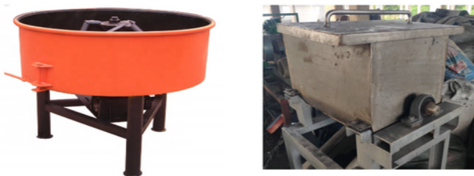
Figure 3.8: Mixing machine - wheel mixer (left) and horizontal mixer (right)
