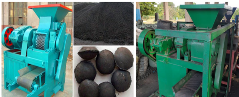
Figure 2.5: Roller press briquetting machine (making oval briquettes)
