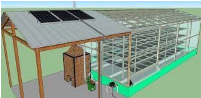
Figure 3.4: Solar-Biomass hybrid drying system machine with carbonized coconut shells crushed
