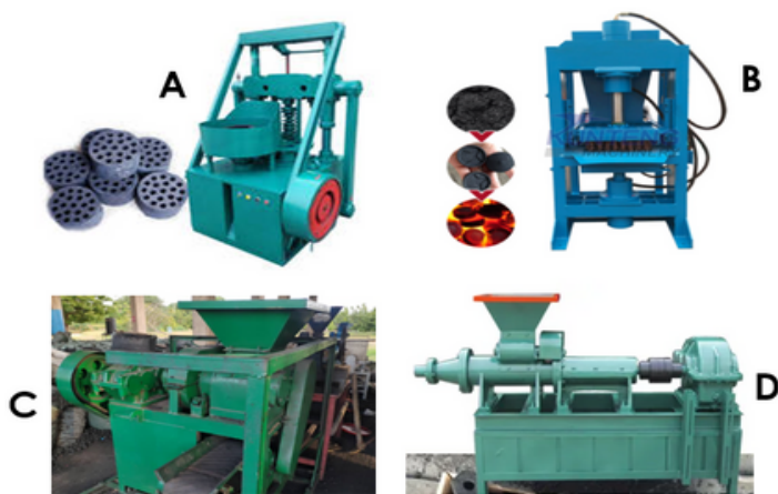
Figure 3.9: Biomass briquette machine including piston press (A), Hydraulic press (B), Roller press (C) and Screw extruder.
